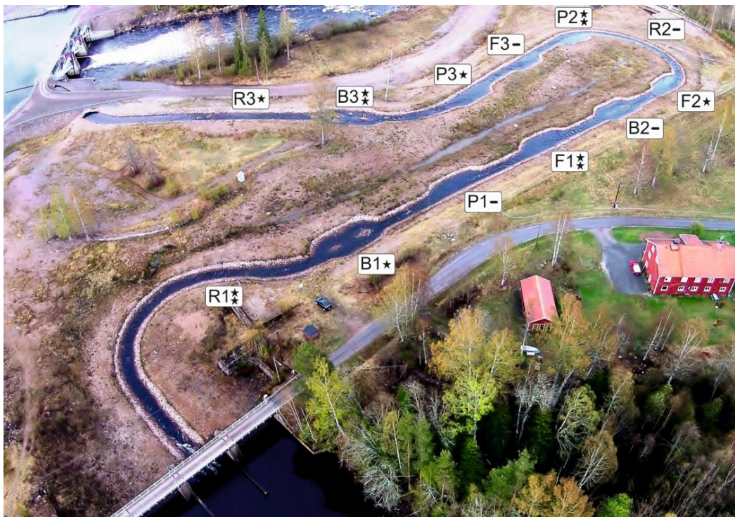
Figure 3. The biocanal before modifications of the channel. Abbreviations; R = riffle, B = braided, P = pool, F = floodplain. – indicates habitats in which no LWD was added, one star indicates habitats in which a low density of LWD later was added and two stars indicates habitats in which a high density of LWD later was added. Photo: Anders Bruks
