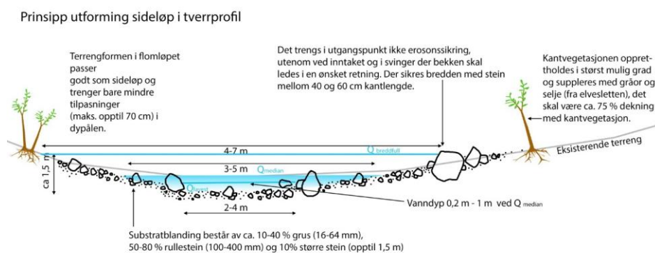
Figure 5 Principle drawing of design and bottom substrate for river wedge in cross profile. Width and depth can be adapted to the natural conditions in the old wedge.
